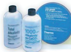
**Total Alkalinity Test Kit:** A two-step direct measurement of total alkalinity and pH. Calibrate for pH, add alkalinity reagent and read total alkalinity of 0-200 ppm CaCO<sub>3</sub> from the included pH conversion chart.
